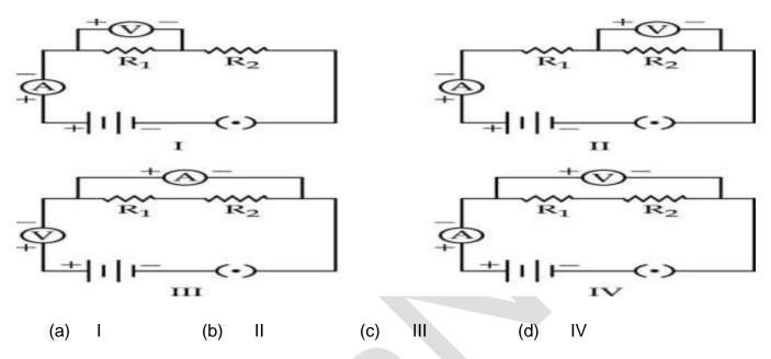
36. In the experiment 'To find the equivalent resistance of two resistors, connected in parallel' two students connected the ammeter in two different ways as shown in the given circuits I and II. The ammeter has been correctly connected in :
