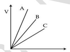
Ohm's law experiment is performed separately with individual resistors  $R_1$ ,  $R_2$  [ $R_1 > R_2$ ] and series combination of  $R_1$ ,  $R_2$ . Graph is plotted between potential difference (V) and current (I) as shown in figure for each case:
