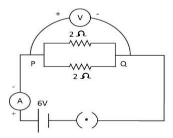
While performing the experiment to find equivalent resistance of a combination of resistances in the circuit shown above; Reena measured reading of voltmeter 'V' which gives potential differences between P and Q. She should find the reading to be:
